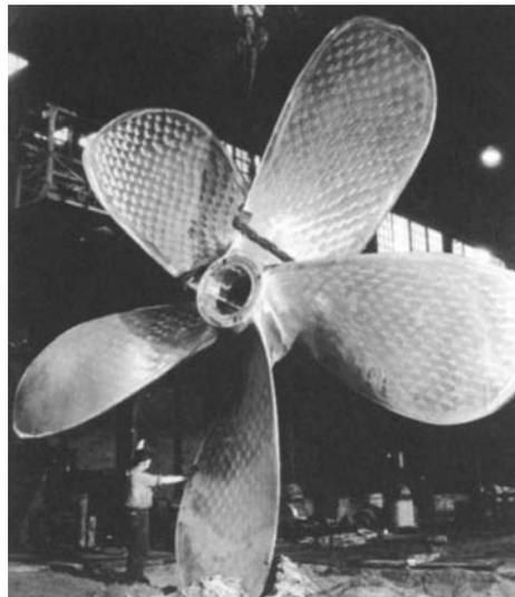
**Fig. 6** Propeller for a 114,000 ton tanker measures 7.5 m (24.7 ft) in diameter and weighs 37.52 Mg (82,725 lb). Part was machined and polished from a single 53.75 Mg (118,500 lb) nickel-aluminum bronze casting.
