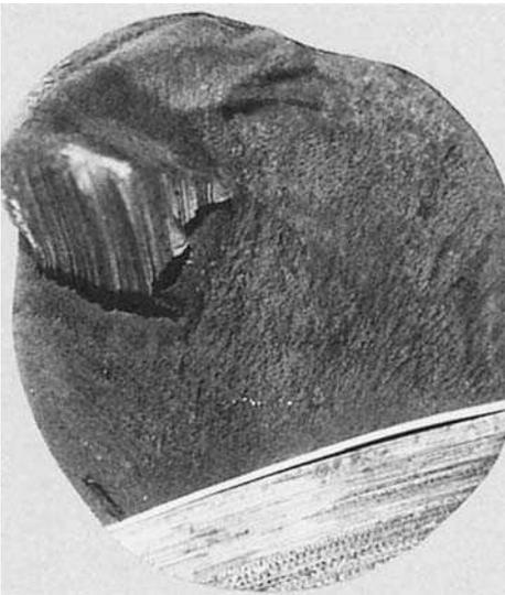
**Fig. 40** Alloy C36000 (free-cutting brass) extrusion. Transverse fracture shows internal cracks, which are associated with a pipe, or extrusion, defect. See also Fig. 41. Not polished, not etched. 1.4 $\times$
