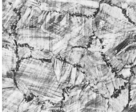
**Fig. 14** C17200 alloy strip, solution annealed and aged at 370 °C (700 °F) for 6 h to attain an overaged condition. The structure shows  $\gamma$  precipitates in the grain boundaries, which appear as dark nodules in a light matrix. Etchant 1 (Table 1). 400 $\times$
