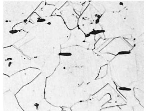
**Fig. 40** Same as Fig. 38, extruded rod. Longitudinal section showing equiaxed grains and dispersed Cu<sub>2</sub>O (dark dots). Etchant 4, Table 3. 400×
