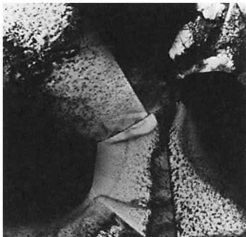
**Fig. 108** Transmission electron micrograph of a rapidly solidified Cu-5Ni-2.5Ti alloy, hot extruded at 750 °C (1380 °F), solution heat treated 1 h at 950 °C (1740 °F); air cooled. Fine precipitate is  $(\text{Cu,Ni})_3\text{Ti}$ . As-polished. 18,000×
