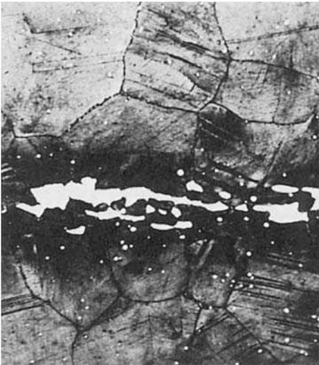
**Fig. 16** C17200 alloy strip, solution annealed and age hardened. The white constituents of the structure are  $\beta$  stringers. These zones of beryllium segregation are carried through from billet casting and homogenization. Etchant 1 (Table 1). 700 $\times$
