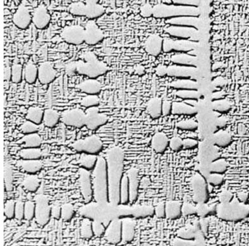
**Fig. 18** Alloy C26000 (cartridge brass), cast, slowly cooled, and quenched. Primary dendrites aligned in (100) crystallographic directions. The fine, quenched structure has the same orientation as the coarse dendrites. Etchant 1, Table 3, then electropolished with electrolyte 1, Table 2. 30×. (J. Dibee)
