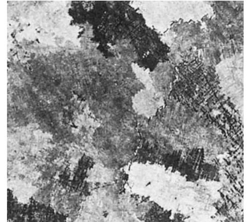
**Fig. 27** Same alloy and processing as Fig. 24, showing fine intergranular cracks in the region of equiaxed grains at the center of the ingot.  $\text{HNO}_3 + \text{H}_2\text{O}$  at 60  $^\circ\text{C}$  (140  $^\circ\text{F}$ ). 4 $\times$
