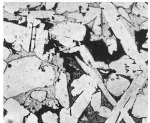
**Fig. 103** Dealuminized alloy C95400 (aluminum bronze), as sand cast. Voids (black) and matrix (medium gray) around  $\alpha$  grains at top resulted from dealuminizing in salt water. Small, gray rosettes in grains are an aluminum-rich aluminum-nickel-iron phase. Alpha grains at the bottom are a matrix of eutectoid transformed  $\beta$  phase. Etchant 8, Table 3. 250 $\times$
