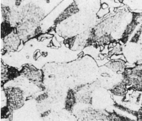
**Fig. 95** Alloy C67500 (manganese bronze A) extruded rod. Iron-rich phase (light, outlined) within  $\beta$  phase (smooth etching) and between  $\alpha$  and  $\beta$  phases. Etchant 1, Table 3. 875 $\times$
