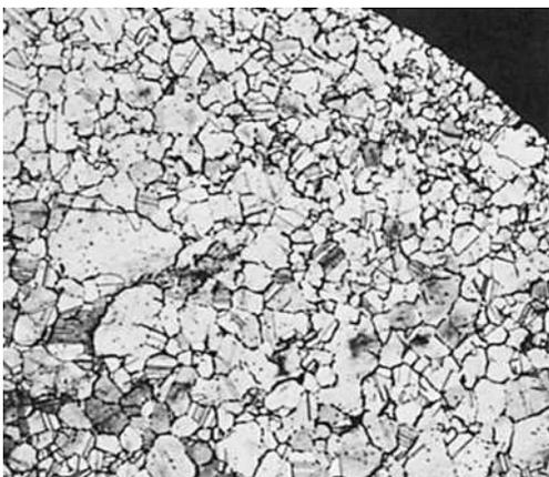
**Fig. 41** Same as Fig. 38, heated in hydrogen. Hydrogen diffused into the copper, reacted with Cu<sub>2</sub>O at the grain boundaries, formed steam, and forced the copper grains apart, causing embrittlement and porosity. See also Fig. 42. Etchant 4, Table 3. 75×
