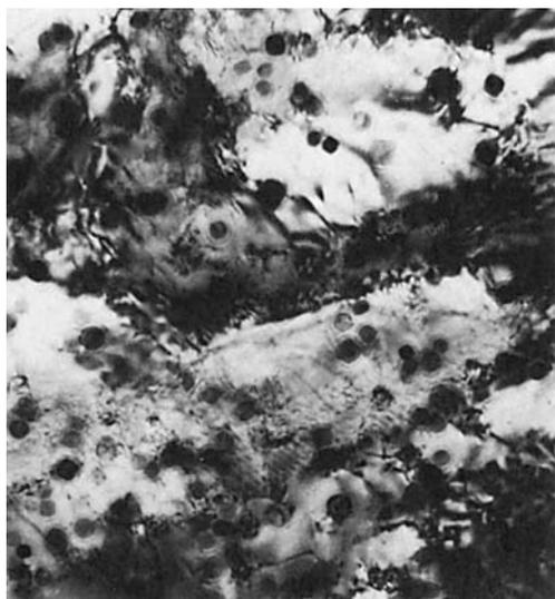
**Fig. 110** Transmission electron micrograph of same alloy and processing as Fig. 109, but higher magnification shows the very fine ( $\sim 0.25 \mu\text{m}$ ) aging precipitate of  $(\text{Cu,Ni})_3\text{Ti}$ . See also Fig. 108 and 109. As-polished. 75,200×
