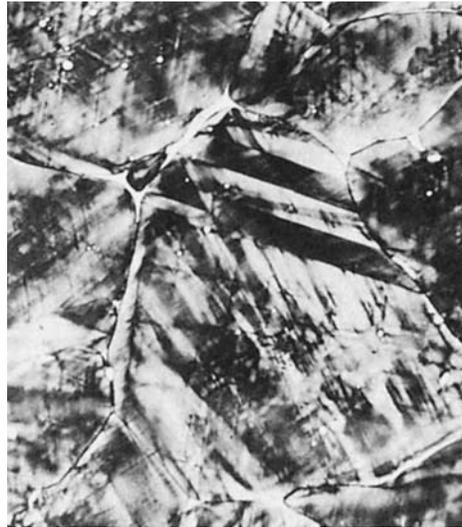
**Fig. 17** C17200 alloy strip heated to 885 °C (1625 °F) and water quenched. The microstructure shows "burned metal" caused by solution annealing at too high a temperature. Partial melting at the grain boundaries, caused by extreme temperatures, resolidifies as  $\beta$  phase. Etchant 1 (Table 1). 700 $\times$
