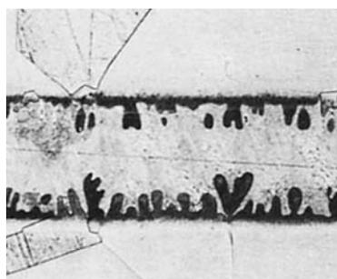
**Fig. 57** Same as Fig. 56, brazed with BAg-8a filler metal. Silver-copper eutectic (mottled gray) in the joint, with small dendrites of copper solid solution (dark) extending into the joint from the unalloyed base metal. Grains of unalloyed copper in the base metal are extremely large. Etchant 5, Table 3. 70×
