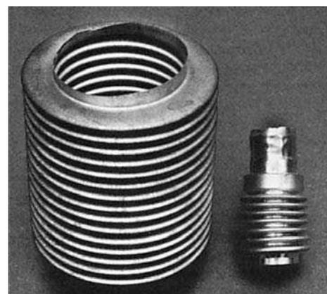
**Fig. 6** Deep-drawn and corrugated copper alloy bellows
