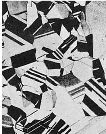
**Fig. 76, 77** Alloy C26000 (cartridge brass) hot rolled to 10 mm (0.4 in.) thick, annealed to a grain size of 15  $\mu\text{m}$ , cold rolled to 40% to 6 mm (0.24 in.) thick, and annealed to a grain size of 120  $\mu\text{m}$ . Diagram in lower left corner of each micrograph indicates the view relative to the rolling plane of the sheet. Nominal tensile strength of 296 MPa (43000 psi). Etchant 1, Table 3. 75×
