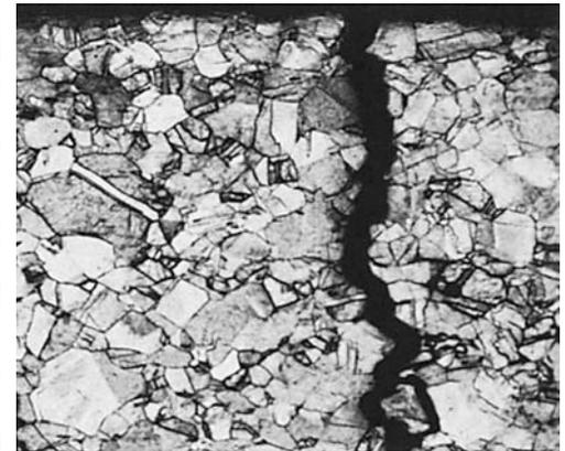
**Fig. 69** Alloy C26000 (cartridge brass) tube, drawn, annealed and cold-reduced 5%. Typical intergranular stress-corrosion crack, with some branching.  $\text{NH}_4\text{OH} + \text{H}_2\text{O}_2$ . 150×
