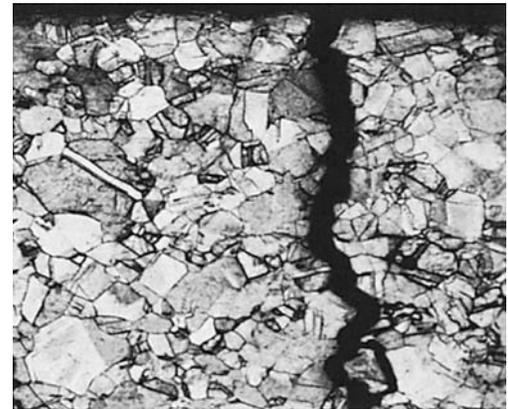
**Fig. 69** Alloy C26000 (cartridge brass) tube, drawn, annealed and cold-reduced 5%. Typical intergranular stress-corrosion crack, with some branching.  $\text{NH}_4\text{OH} + \text{H}_2\text{O}_2$ . 150×
