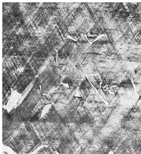
**Fig. 2** C82500 alloy casting, solution annealed at 790 °C (1450 °F) and aged to peak hardness at 315 °C (600 °F) for 3 h. Microstructure consists of Chinese-script beryllides in a copper-rich  $\alpha$  solid-solution matrix, with angular  $\beta$  phase transformed to a lamellar aggregate of  $\alpha$  and  $\gamma$  phases. Striations are the result of metastable precipitation in the alloy. Etchant 1 (Table 1). 400 $\times$
