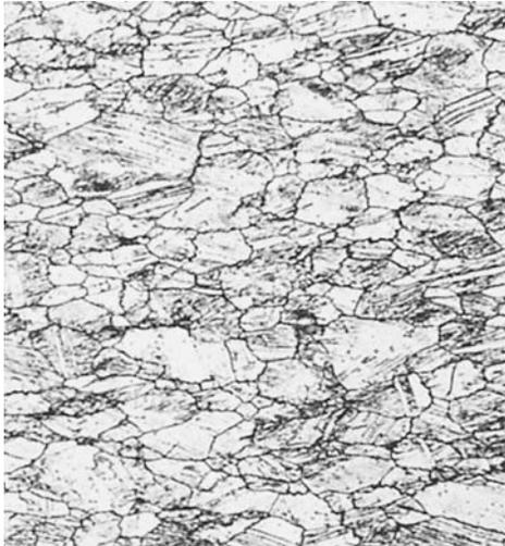
**Fig. 4** C17200 alloy strip, mill hardened to XHMS (TM08) temper for high strength and limited formability. Longitudinal section shows elongated grains of the  $\alpha$  phase and cobalt beryllides. Striations result from precipitation of metastable phases not resolved by optical microscopy. Etchant 1 (Table 1). 400 $\times$
