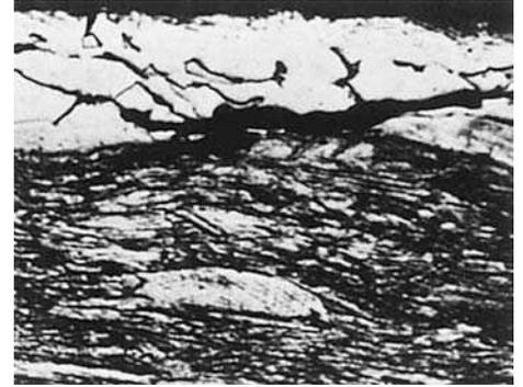
**Fig. 39** Phosphor bronze strip rolled from a static-cast ingot, showing gross tin sweat on the surface (top). Illustrates how segregation caused by exudation persists in the fabricated structure. Etchant not reported. 300 $\times$ . Source: Ref 34
