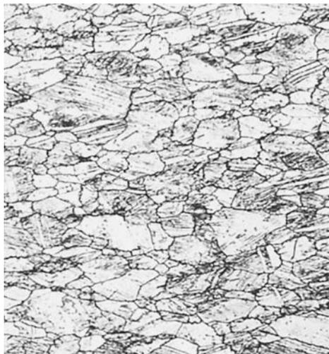
**Fig. 4** C17200 alloy strip, mill hardened to XHMS (TM08) temper for high strength and limited formability. Longitudinal section shows elongated grains of the  $\alpha$  phase and cobalt beryllides. Striations result from precipitation of metastable phases not resolved by optical microscopy. Etchant 1 (Table 1). 400 $\times$
