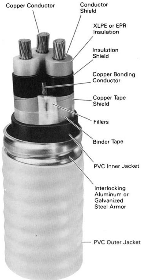
**Fig. 5** Armored power cable as used in mines and industrial applications. EPR, ethylene propylene rubber. Source: Ref 14
