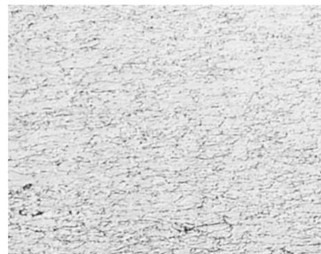
**Fig. 12** C17500 alloy strip, solution annealed, cold rolled, and precipitation hardened at 480  $^{\circ}\text{C}$  (900  $^{\circ}\text{F}$ ) for 2 h to achieve maximum hardness. Structure consists of the  $\alpha$  phase and a uniform distribution of the beryllide phase. Elongated grains are the result of cold work, and metastable hardening precipitates are not resolved. Etchant 6 (Table 1). 400 $\times$
