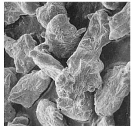
**Fig. 26** Scanning electron micrograph of prealloyed, air-atomized bronze (89%Cu-9%Sn-2%Zn). 165×
