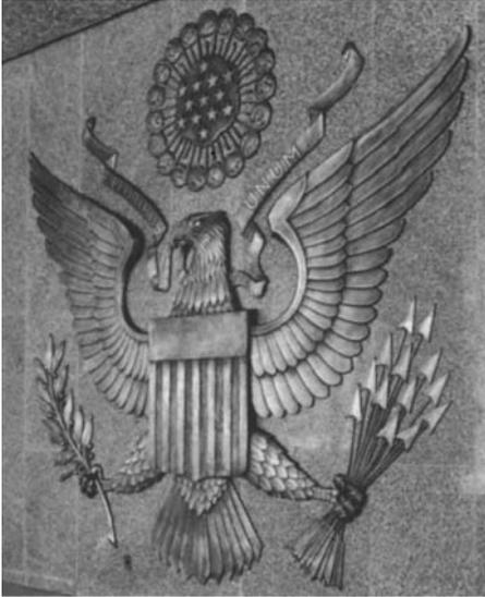
**Fig. 8** Twelve-foot-high bronze sand casting of the Great Seal of the United States located in lobby of the Federal Deposit Insurance Corporation building in Washington, D.C. Weight, 1.8 Mg (4000 lb)
