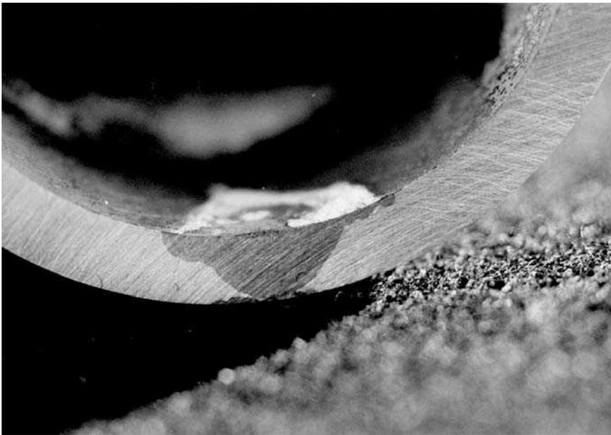
**Fig. 5** A large plug of dezincified metal beneath a deposit on a brass pipe
