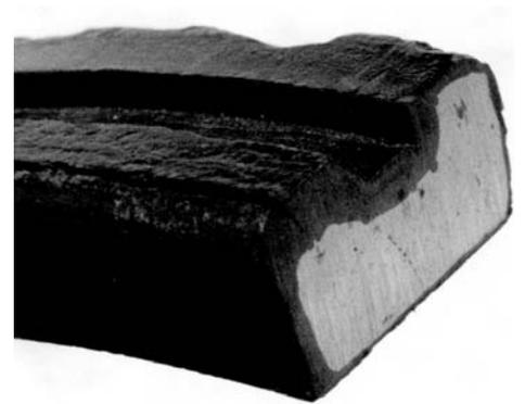
**Fig. 7** Layer-type dezincification of a brass pump component. The dark (red) outer layers are uniformly corroded regions surrounding the uncorroded metal (original yellow) of the brass.
