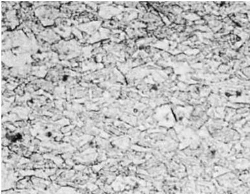
**Fig. 116** Temper: half hard (H02). Moderately cold-worked, fine-grained structure
