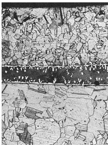
**Fig. 59** Brazed joint between tubes of copper C12200 (DHP copper). Filler metal was BAg-1. See Fig. 61 for details of structure. Etchant 4, Table 3. 75×
