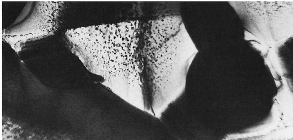
**Fig. 109** Transmission electron micrograph of same alloy as in Fig. 108, solution heat treated at 950 °C (1740 °F) for 1 h and air cooled. Grain size is less than 2  $\mu\text{m}$ . The structure is primary  $\text{Ni}_3\text{Ti}$  and a fine precipitate of  $(\text{Cu,Ni})_3\text{Ti}$ . See also Fig. 108 and 110. As-polished. 28,000×
