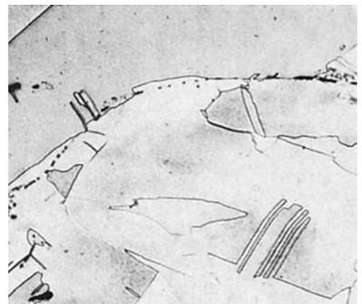
**Fig. 43** Copper C12500 (FRTP copper) hot-rolled strip 12.7 mm (0.5 in.) thick. Structure consists of twinned grains of copper, with stringers of Cu<sub>2</sub>O particles resulting from segregation of the oxide in the ingot during casting. Etchant 1, Table 3. 200×
