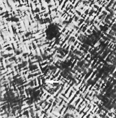
**Fig. 12** Transmission electron micrograph of spinodal microstructure developed in a 66.3 Cu-30Ni-2.8Cr (wt%) alloy during slow cooling from 950 °C (1740 °F). The microstructure is homogenous up to the grain boundary indicated by the arrow. 35,000×
