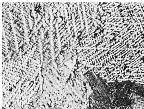
**Fig. 15** Alloy C68700 (arsenical aluminum brass), as-cast. Macrosection showing typical dendritic structure. See Fig. 16 for detail. Etchant 18, then etchant 16, Table 3. 4 $\times$ . (J. Dibee)
