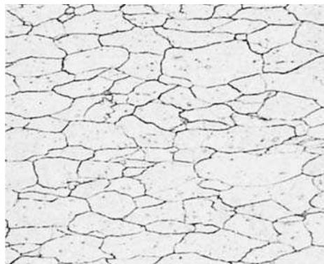
**Fig. 8** C17200 alloy strip, solution annealed at 790  $^{\circ}$ C (1450  $^{\circ}$ F) and cold rolled at 37% to full hard temper. Longitudinal section shows elongated grains of  $\alpha$  phase and cobalt beryllides. Etchant 1 or 2 (Table 1). 400 $\times$
