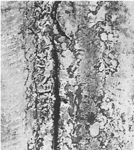
**Fig. 24** Alloy C36000 (free-cutting brass) semicontinuous cast in a 254 mm (10 in.) diam ingot. A longitudinal crack in the surface of the ingot. Severe macrosegregation can accompany cracks of this type. See also Fig. 39. Not polished, not etched. Actual size
