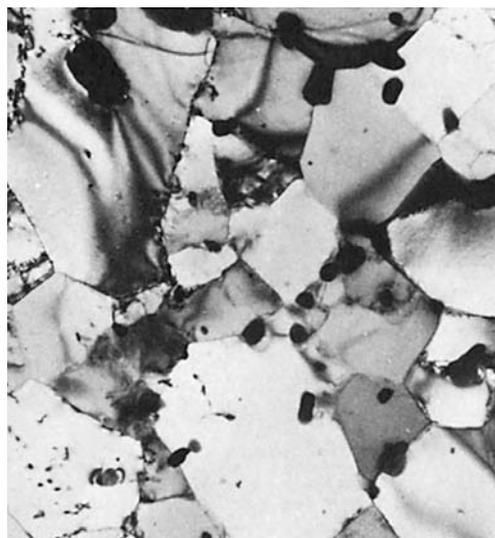
**Fig. 111** Transmission electron micrograph of a copper-zirconium (0.57Zr, with 0.31ZrO<sub>2</sub>) powder metallurgy product, as hot extruded. The relatively coarse dark particles are  $\text{Cu}_5\text{Zr}$  precipitates; the finer dark particles are probably  $\text{ZrO}_2$ . As-polished. 24,480×. (N. Grant)
