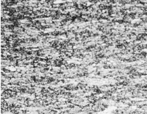
**Fig. 113** Temper: spring (H08). Elongated, cold-worked, fine-grained structure
