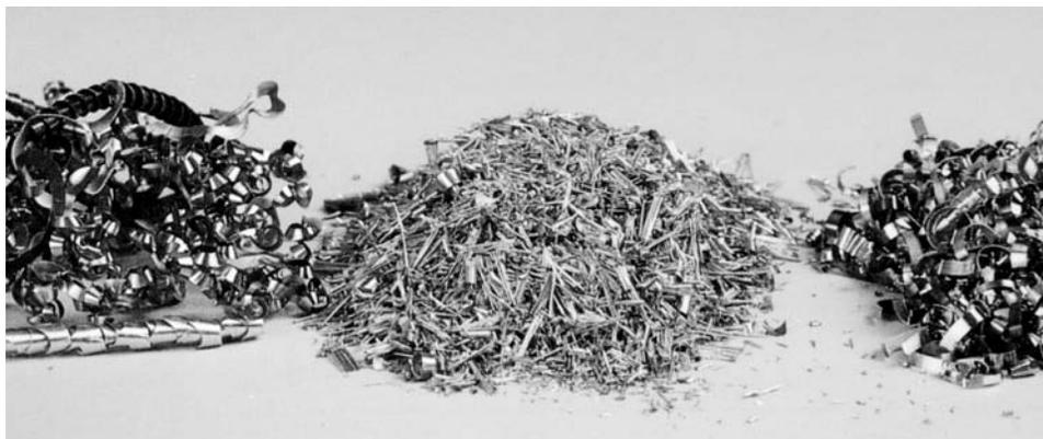
**Fig. 4** Broken chips typical of free-cutting brass, type I (center), flanked by type II, short-chip turnings (right), and type III, long-chip turnings (left)
