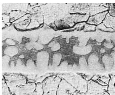
**Fig. 56** Copper C10100 (OFE copper) brazed with BCuP-5 filler metal. Silver-copper-phosphorus eutectic (mottled gray) in the joint, with large dendrites of copper solid solution (light gray) extending into the joint from the grains of unalloyed base metal. Grains of unalloyed copper in the base metal are medium size. Compare with Fig. 53. Etchant 5, Table 3. 125×
