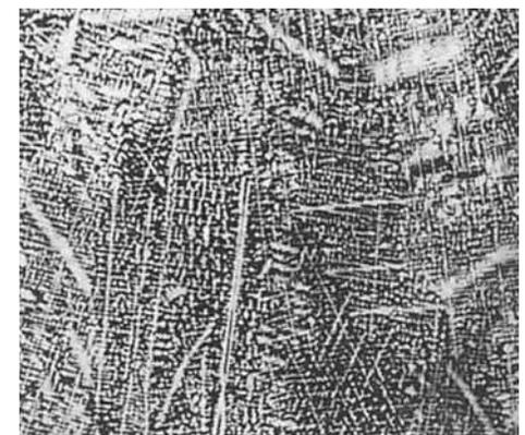
Fig. 5 Alloy C71500 (copper nickel, 30%) ingot. Dendritic structure in the columnar region of the ingot shows coring (variation in solute concentration). The light areas are nickel-rich; the dark areas are low in nickel. Waterbury reagent. 20x
