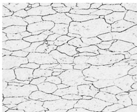
**Fig. 8** C17200 alloy strip, solution annealed at 790  $^{\circ}\text{C}$  (1450  $^{\circ}\text{F}$ ) and cold rolled at 37% to full hard temper. Longitudinal section shows elongated grains of  $\alpha$  phase and cobalt beryllides. Etchant 1 or 2 (Table 1). 400 $\times$
