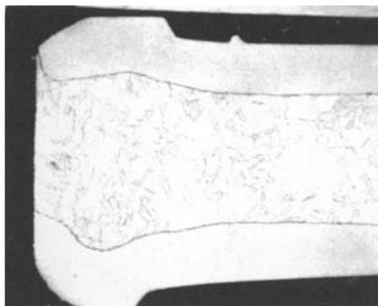
**Fig. 4** Metallographic cross section of the edge of a cupronickel-clad copper coin.
