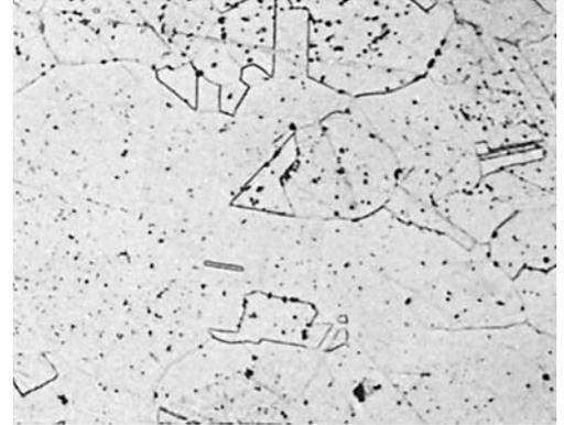
**Fig. 37** Same as Fig. 35, hot-rolled bar, heated 1 h in air to 665 °C (1225 °F). Specimen from near surface shows Cu<sub>2</sub>O (dark dots) caused by oxygen penetration during heating. Etchant 1, Table 3. 250×
