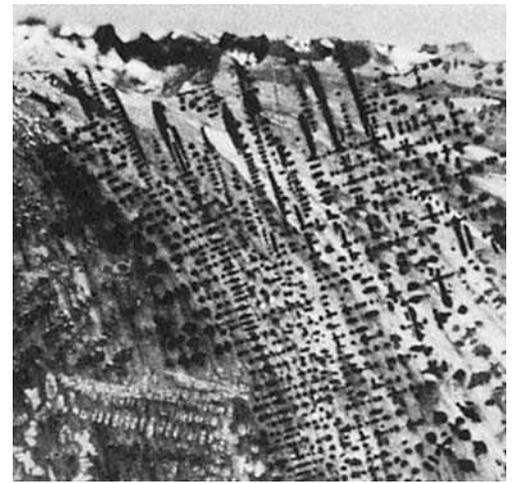
**Fig. 1** Alloy C11000 (ETP copper), static cast. Excellent definition of dendritic structure. Etchant 10, Table 3. 5 $\times$ . (J. Bartholomew)
