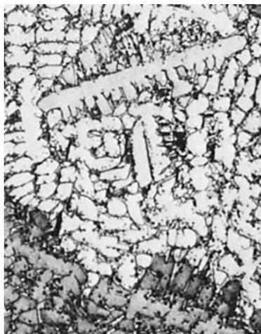
**Fig. 7** Same material as Fig. 6, with primary dendrites of  $\alpha$  phase darkened. Lead appears as small spheroids. Etchant 1, Table 3. 50 $\times$ . (J. Dibee)
