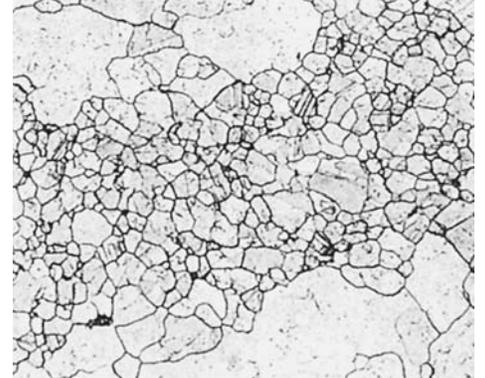
**Fig. 15** C17200 alloy plate, cast, homogenized, and hot worked. The microstructure shows nonuniform distribution of grain sizes, which is typical of a hot-worked product. Greater uniformity in grain size distribution may be achieved in the finished product by successive cold-working and annealing operations. Etchant 1 (Table 1). 700 $\times$
