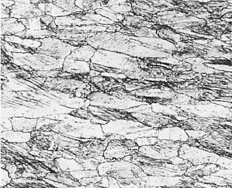
**Fig. 13** C17200 alloy strip, solution annealed, cold rolled full hard, and precipitation hardened at 315 °C (600 °F) for 2 h to achieve maximum hardness. Longitudinal section shows elongated grains of  $\alpha$  phase and cobalt beryllides. Striations are caused by metastable precipitates not resolved by optical microscopy. Etchant 1 (Table 1). 400 $\times$
