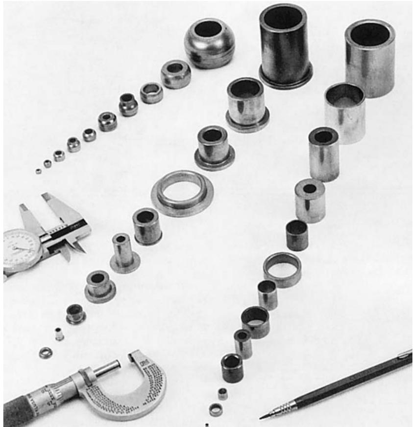
**Fig. 6** Typical bronze self-lubricating bearings. The most common shapes are simple or flanged bushings, but some have spherical external surfaces. Sizes range from about 0.8 to 75 mm ( $1/32$  to 3 in.).
