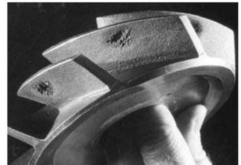
**Fig. 4** Cavitation damage repeated on successive vanes of a bronze impeller
