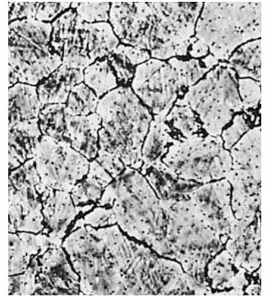
**Fig. 50** Same alloy and processing as Fig. 49, but aged 3 h at 360  $^{\circ}C$  (600  $^{\circ}F$ ) after solution treatment. Typical hardness is 37 HRC. Copper-beryllium precipitate at grain boundaries and within  $\alpha$  grains. Etchant 3, Table 3. 300 $\times$
