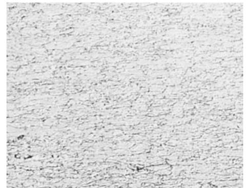
**Fig. 12** C17500 alloy strip, solution annealed, cold rolled, and precipitation hardened at 480  $^{\circ}$ C (900  $^{\circ}$ F) for 2 h to achieve maximum hardness. Structure consists of the  $\alpha$  phase and a uniform distribution of the beryllide phase. Elongated grains are the result of cold work, and metastable hardening precipitates are not resolved. Etchant 6 (Table 1). 400 $\times$
