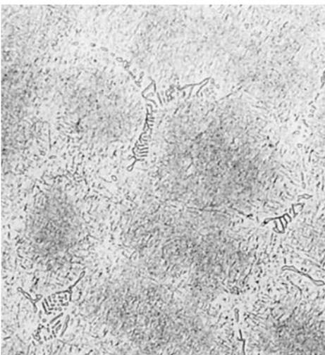
**Fig. 1** C82200 alloy casting. As-cast microstructure shows interdendritic networks of large primary beryllide phase in a matrix of  $\alpha$  solid solution. Preferred orientation of small secondary beryllides is observed with the matrix. Etchant 6 (Table 1). 400 $\times$
