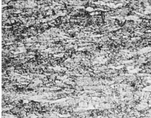
**Fig. 114** Temper: extra hard (H06). Elongated, cold-worked, fine-grained structure
