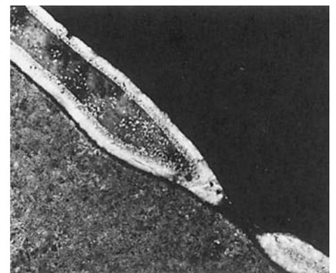
**Fig. 36** Alloy C36000 (free-cutting brass) ingot, semicontinuous cast. Zinc-rich "smudges" on the surface (top left to bottom right) are the result of condensation, on the mold wall, of zinc vapor trapped by the layer of carbon powder covering the melt. This problem has been solved by the use of proprietary glass covers that prevent zinc evaporation and recondensation. NH<sub>4</sub>OH + H<sub>2</sub>O<sub>2</sub>. 10 $\times$
