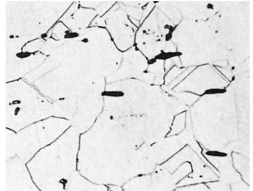
**Fig. 40** Same as Fig. 38, extruded rod. Longitudinal section showing equiaxed grains and dispersed Cu<sub>2</sub>O (dark dots). Etchant 4, Table 3. 400×
