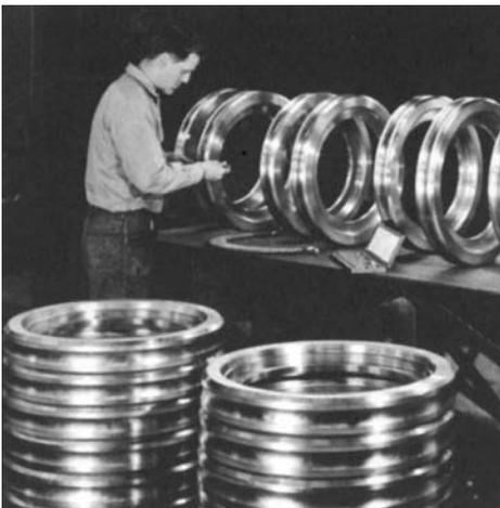
**Fig. 5** Centrifugally cast aluminum bronze worm gear blanks being inspected
