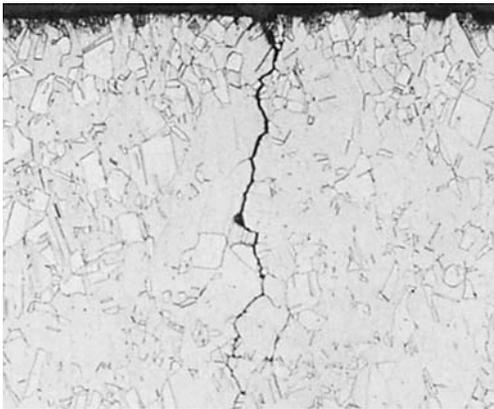
**Fig. 67** Copper C12200 drawn condenser tube, with a branched intergranular stress-corrosion crack starting at an outside surface. See Fig. 68 for details of a similar crack. Potassium dichromate. 100×
